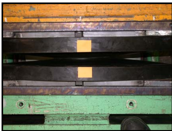
Figure 2: RoGlider ready for testing Displacement 0\text{mm} , vertical force of 850\text{kN}
