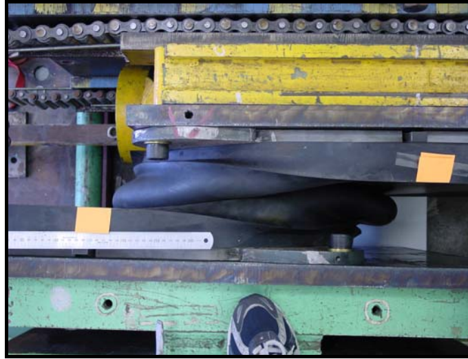
Figure 4: RoGlider during Test Displacement +575mm, vertical force of 110kN
