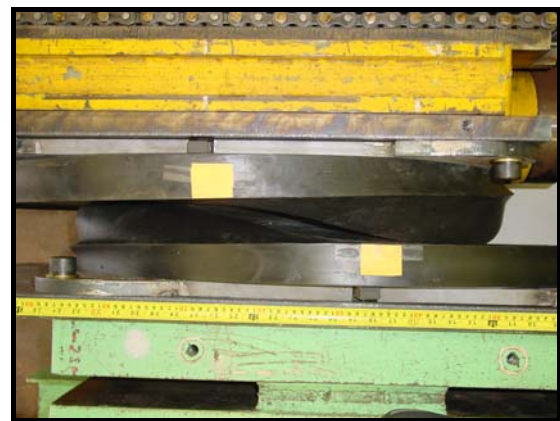
Figure 3: RoGlider during Test Displacement -150\text{mm} , vertical force of 850\text{kN}
